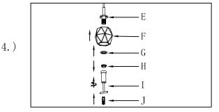
Step.4: Install Glass(F)/Cap(G) onto socket(E). Install socket ring(H) onto socket (E) by spanner (I). Then install G9 LED bulb (J) into socket(E).
