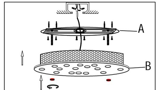
Step.3: Install canopy (B) to bracket (A) and tighten finials until flush with the ceiling.
