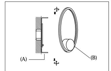
Step 3: Install Body (B) to Canopy (A) and tighten screws on the sides of the canopy to secure.
