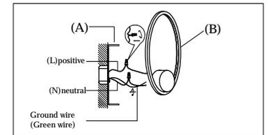
Step 2: Wire fixture to wires in outlet box. Install Green wire to Ground Screw.
