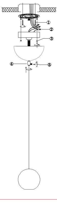
WARNING: Wires need to be connected to driver found in canopy and should not connect directly to power source or a short might occur.
