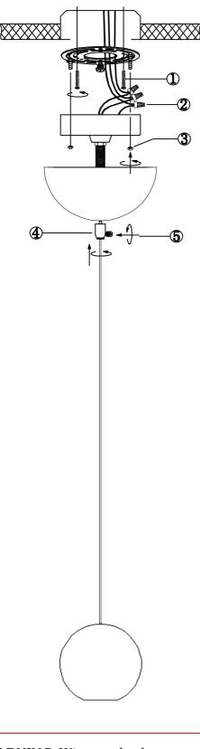
WARNING: Wires need to be connected to driver found in canopy and should not connect directly to power source or a short might occur.
