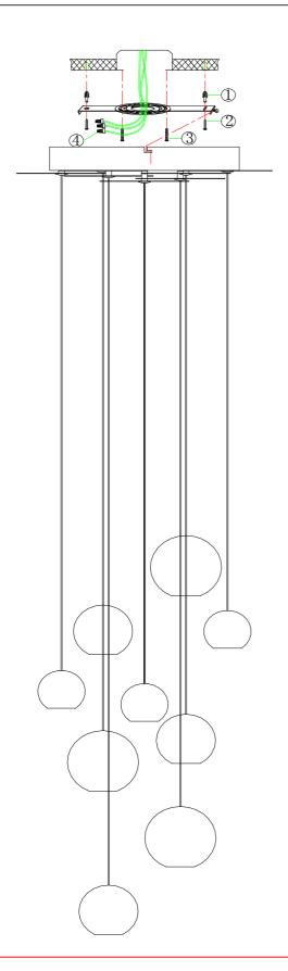
WARNING: Wires need to be connected to driver found in canopy and should not connect directly to power source or a short might occur.
