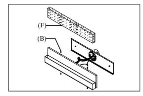
Step 2: Then wire fixture to wires in outlet box. Copper wire is for Ground. Install lamp body to mounting bracket using two screws on side.
