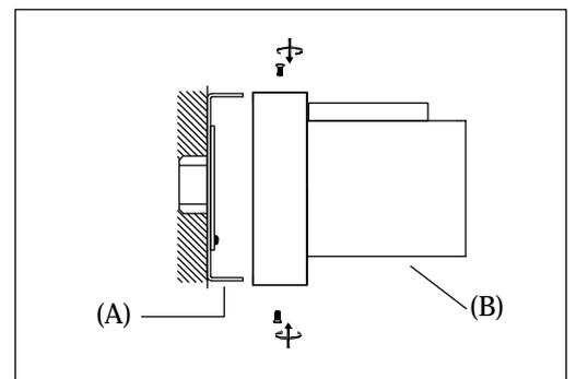
**Step.3: Install Body (B) to Canopy (A) and tighten screws at the ends of the canopy to secure.**
