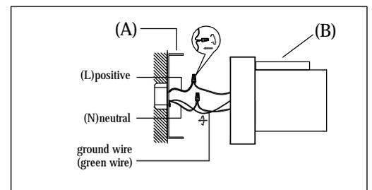
**Step.2: Wire fixture to wires in outlet box. Install Green wire to Ground Screw.**
