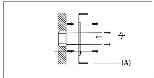
**Step.1: Remove Bracket (A) from fixture and install to electrical box.**
