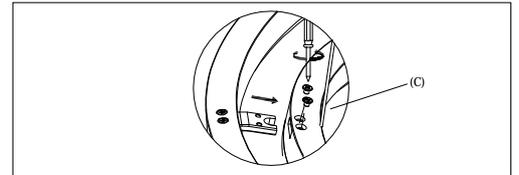
**Step.1:** First connect the lamp body (C) parts together by inserting male tab at opening and screw to secure.
