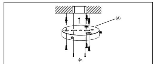
**Step.2:** Remove Bracket (A) from fixture and install to electrical box.
