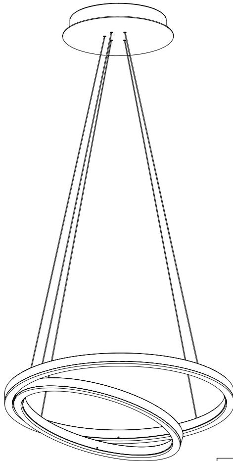
**WARNING: WIRES NEED TO BE CONNECTED TO DRIVER FOUND IN CANOPY AND SHOULD NOT CONNECT DIRECTLY TO POWER SOURCE OR A SHORT MIGHT OCCUR.**
