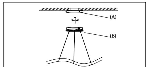
**Step 4:** Adjust wire length to desired hanging height. Install Canopy (B) to Bracket (A) and tighten screws at the ends of canopy to secure.
