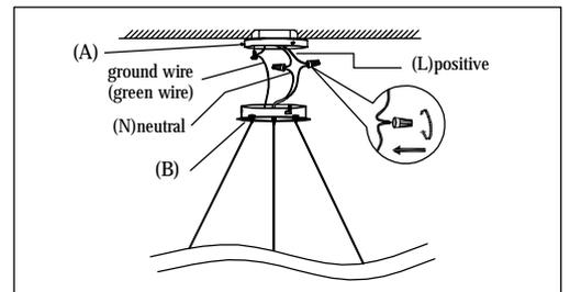
**Step.3:** Wire fixture to wires in outlet box. Install Green wire to Ground Screw.
