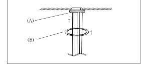
Step 4: Adjust wire length to desired hanging height. Install Canopy (B) to Bracket (A) and tighten screws at the ends of canopy to secure.
