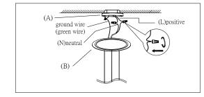
Step.3: Wire fixture to wires in outlet box. Install Green wire to Ground Screw.
