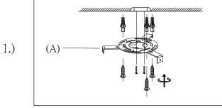
Step.1: Remove Bracket (A) from fixture and install to electrical box.
