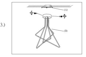
Step 3:Install Body (B) to Bracket (A) and tighten screws at the ends of the canopy to secure.
