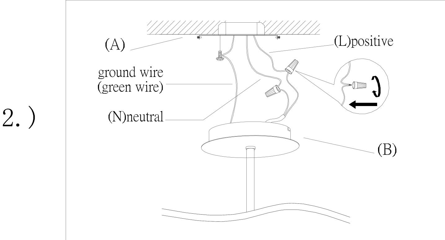
Step 2: Use push pins to adjust wires to desired mounting height. Wire fixture to wires in outlet box. See dual plastic wire instructions for more details. Install Green wire to Ground Screw.
