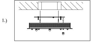
Step.1: Remove mounting bracket (A) from fixture and install to electrical box.
