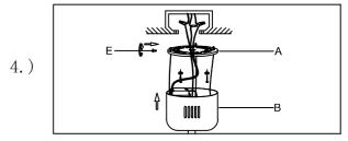
Step.4: Wire fixture to wires in the outlet box. Black wire is live. White wire is neutral. Copper wire is for Ground. Make sure red/black wire is connected to transformer found in the canopy.
