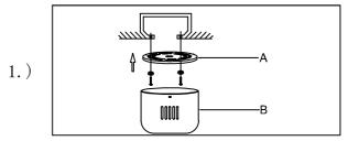
Step.1: Remove mounting bracket from canopy and install to electrical box.
