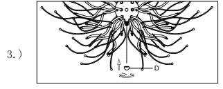
Step.3: Tighten the ball nut (D) on the bottom of the fixture.
