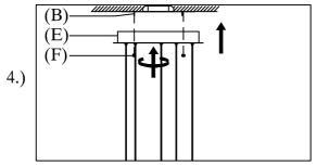
Step4: Install fixture to bracket(B) and Decorative Nuts(F) at the ends of the canopy(E) to secure.
