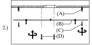
Step2:Remove mounting bracket from fixture and install to electrical box.
