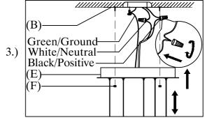
Step3: Adjust wire length to desired mounting height, and tighten strain relief screws to secure. Wire fixture to wires in outlet box. Green wire is for Ground.
