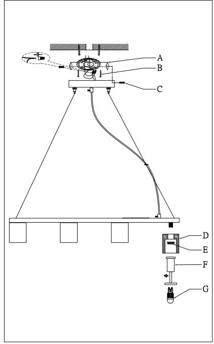
Step.1: Remove mounting bracket (A) and install t electtical box. Mark where anchors meet ceiling, remove mounting bracket from ceiling, and then drill holes using  $\frac{3}{16}$ " drill bit where marked(B). Install mounting bracket and attach anchors to secure bracket at ends.
