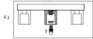
Step.4: Install maximum 2.2W G9LED Xenon bulbs (G) to the socket.
