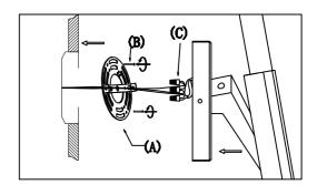
Step 1: Remove mounting bracket (A) from fixture and install to electrical box. Then wire fixture (C) to wires in outlet box. Copper wire is for Ground.
