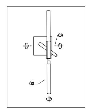
Step 2: Install lamp body to back plate using two screws (D) on the sides. Thread acrylic rod (E) to fixture.
