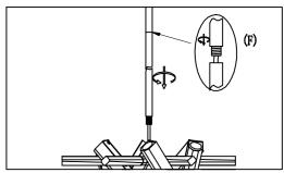
Step 1: Run wire through stems (F) and combine stem lengths to meet desired mounting height.
