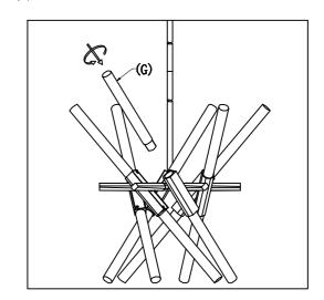
Step 3: Thread acrylic rod (G) onto fixture.
