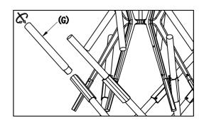
Step 3: Thread acrylic rod (G) onto fixture.
