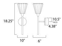
\*Height from center of outlet to top of the fixture
