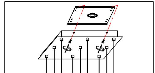
**Step.3: Tighten screws (D) on the sides of the canopy (C) to secure the fixture.**
