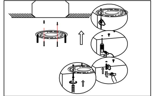
**Step.1: Remove mounting bracket (A) and install to electrical box. Mark where anchors meet ceiling, remove mounting bracket from ceiling, and then drill holes using 3/16" drill bit where marked (B). Install mounting bracket and attach anchors to secure bracket at ends.**
