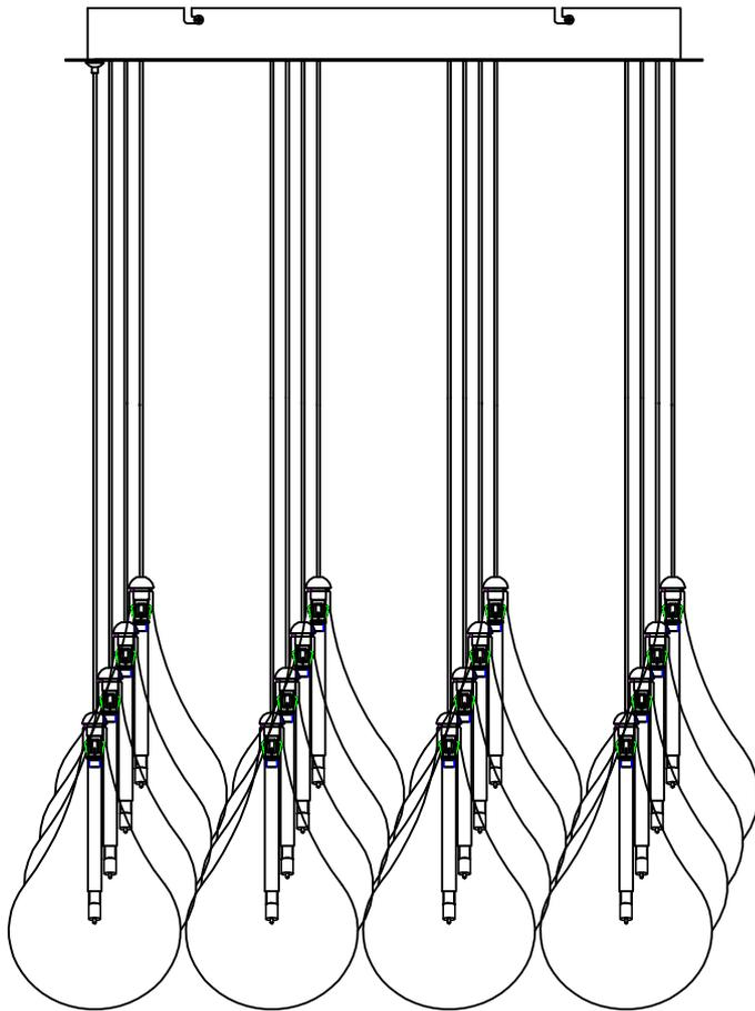
**WARNING:** Wires need to be connected to transformer found in canopy and should not be connected directly to power source or a short may occur
