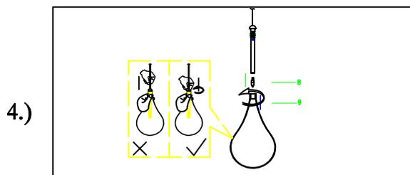
**Step.4: Install G4 bulb (E) provided. Gently turn glass (F) onto socket (D) to secure.**
