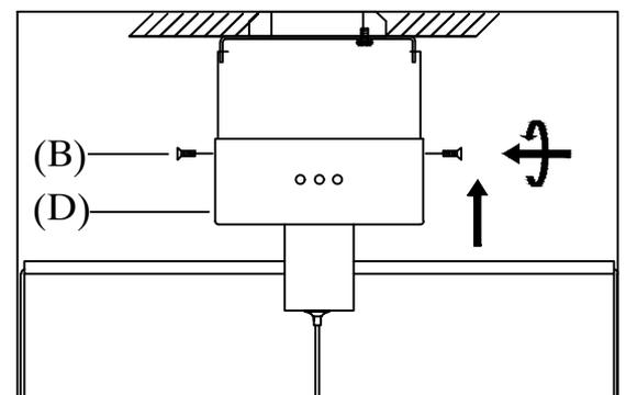
Step3 :Install fixture to bracket and Screws at the ends of the canopy to secure.
