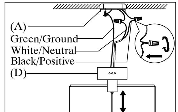
Step2 :Adjust wire length to desired mounting height, and tighten strain relief screws to secure. Wire fixture to wires in outlet box. Green wire is for Ground.
