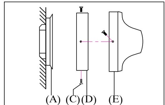
Step3 :Install fixture to bracket and tighten screws at the ends of the Back plate to secure.
