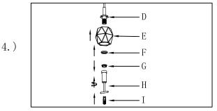
Step.4: Install Glass(E)/Cap(F) onto socket(D). Install socket ring(G) onto socket (D) by spanner (H). Then install G9 LED bulb (I) into socket(D).
