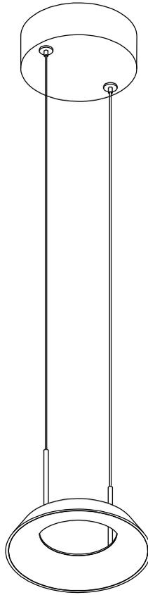
WARNING: WIRES NEED TO BE CONNECTED TO DRIVER FOUND IN CANOPY AND SHOULD NOT CONNECT DIRECTLY TO POWER SOURCE OR A SHORT MIGHT OCCUR.
