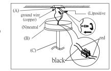
Step.3: Wire fixture to wires in outlet box. Install green wire to ground screw.
