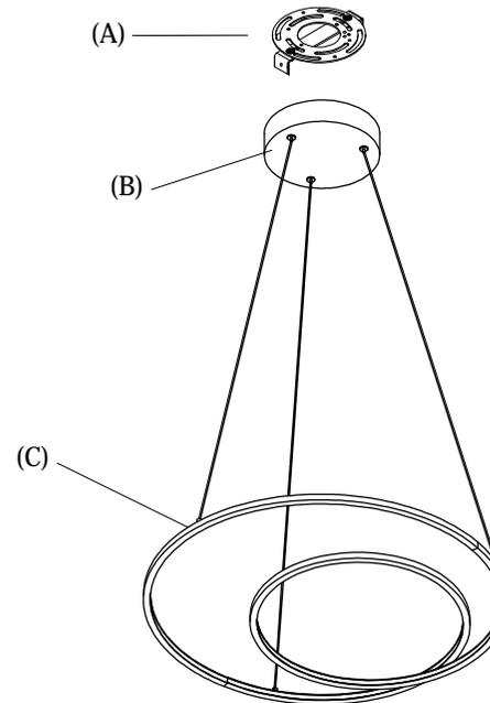
**WARNING: WIRES NEED TO BE CONNECTED TO DRIVER FOUND IN CANOPY AND SHOULD NOT CONNECT DIRECTLY TO POWER SOURCE OR A SHORT MIGHT OCCUR.**
