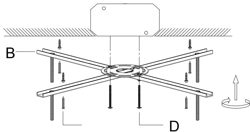
Install mounting bracket (B) to outlet box and attach anchors (C) to secure bracket at ends. Drill holes using  $3/16" \pm$  drill bit where marked.
