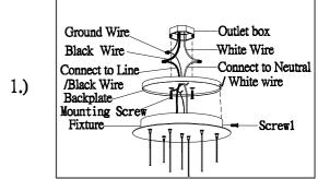
Step.1: Remove backplate from fixture and install to electrical box. Wire fixture to wires in outlet box. Copper wire is for Ground.
