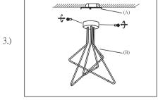
Step 3:Install Body (B) to Bracket (A) and tighten screws at the ends of the canopy to secure.
