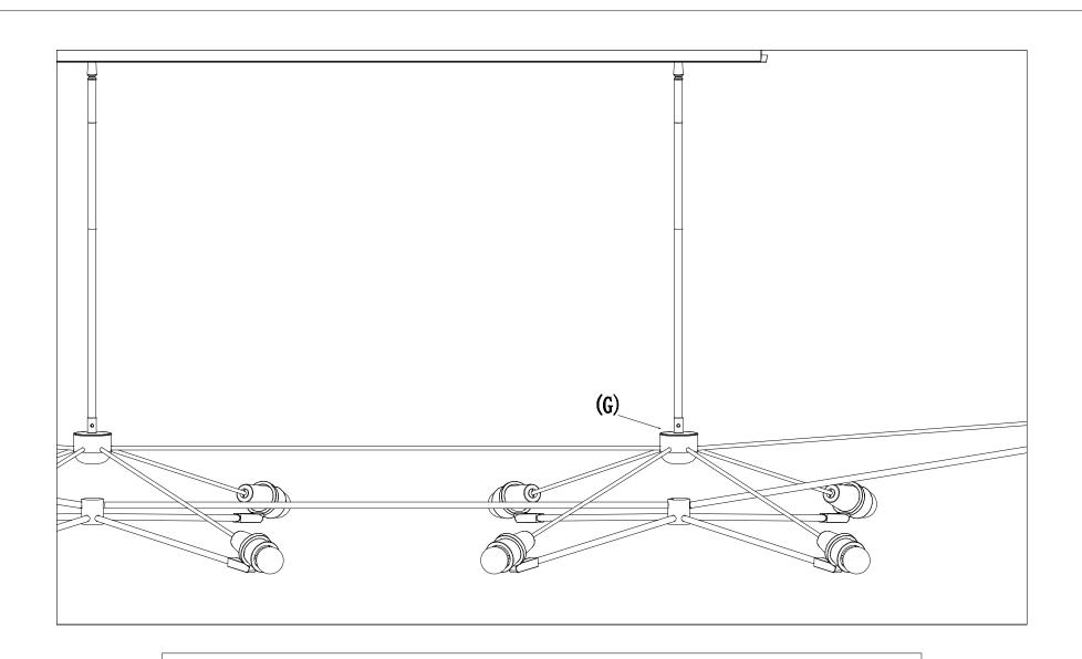
NOTE: Wires can be adjusted within collector(G).
