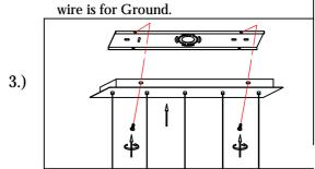
Step. 3: Tighten screws (D) on the sides of the canopy (C) to secure the fixture.
