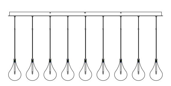
WARNING: Wires need to be connected to transformer found in canopy and should not be connected directly to power source or a short may occur
