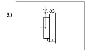
Step.3: Install fixture to bracket and tighten finials (C) at the ends of the canopy to secure.
