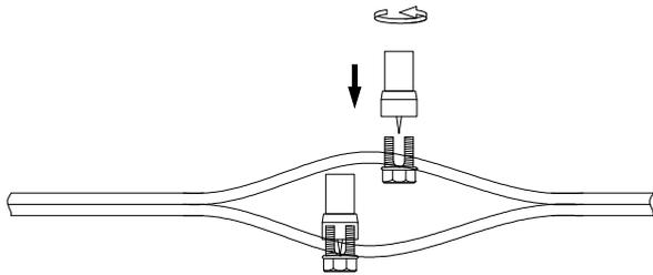
3. Screw the pin into the locking cover to pierce the wire and tighten the large cover.
