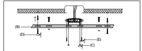
**Step.1:** Remove mounting bracket from fixture and install to electrical box using screws (E). Mark where screws at ends of bracket (B) meet the ceiling. Remove mounting bracket (B) from ceiling. Drill holes using  $3/16" \pm$  drill bit where marked. Install mounting bracket (B) to outlet box by attaching anchors (D) and screw nuts (C) to secure bracket at ends.
