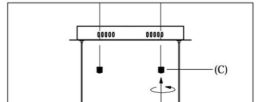
**Step.3:** Adjust wire length to desired mounting height and tighten strain relief screws to secure. Install fixture to bracket and tighten screws (C or F) on the canopy to secure.
