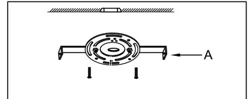
Step.1: Remove Mounting Bracket (A) from Canopy to install to electrical box.
