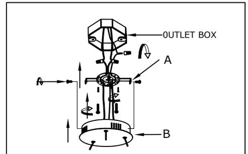
Step.2: Wire fixture to wires in outlet box. Bare wire is for Ground. Secure canopy(B) to mounting bracket using screws on the sides of the canopy.
