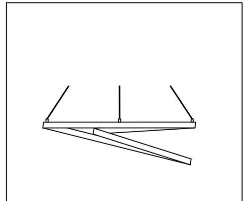
Step.3: Adjust wire length to desired mounting height and fixture configuration
