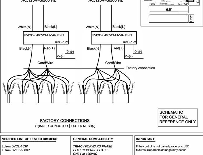
Due to inrush current, wattage should not exceed 150W on a 600W dimmer
