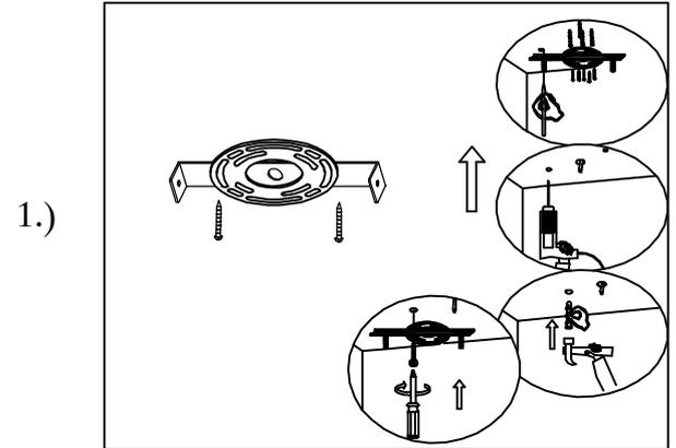
Step.1: Remove mounting bracket (A) and install 1 electrical box. Mark where anchors meet ceiling, remove mounting bracket from ceiling, and then drill holes using  $\frac{3}{16}$ " drill bit where marked (B). Install mounting bracket and attach anchors to secure bracket at ends.
