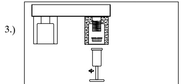
Step.3: Secure the acrylic (D) with the screw ring (E) over the socket and tighten using socket wrench (F)
