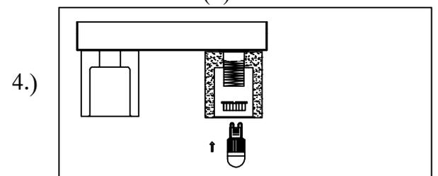
Step.4: Install maximum 2.2W G9LED Xenon bulbs (G) to the socket.
