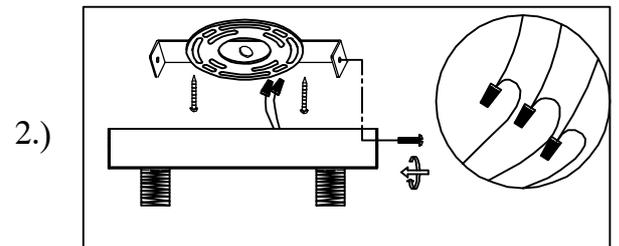
Step.2: Wire fixture to wires in outlet box. Green wire is for Ground. install fixture to the bracket and tighten screws (C) until the fixture is flush with the ceiling.
