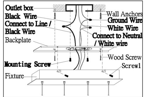
1. Remove mounting bracket (A) from fixture (B) and install to electrical box
