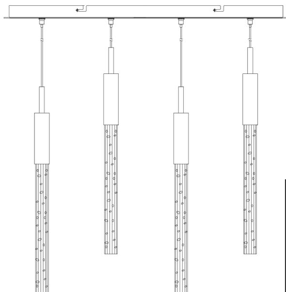
The fixture is designed to dim with a standard Triac forward phase dimmer. Dimming levels will vary by dimmer.
