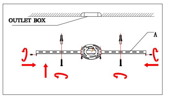
Step.1: Remove mounting bracket from fixture and install to electrical box. Mark where screws at ends of bracket meet the ceiling. Remove mounting bracket from ceiling. Drill holes using 3/16"± drill bit where marked. Install mounting bracket to outlet box and attach anchors to secure bracket at ends.
