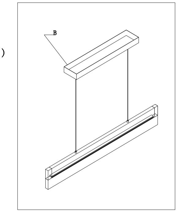
Step.2: Adjust wire length to desired mounting height, and tighten strain relief screws to secure. Wire fixture to wires in outlet box. Install fixture to bracket and tighten screws at the ends of the canopy to secure.
