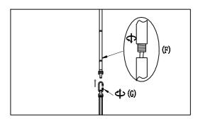
Step 1: Run wire through stems (F) and combine stem lengths to meet desired mounting height. Using carabiner (G) attach fixture to the stems.
