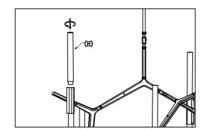
Step 3: Thread acrylic rod (G) onto fixture.
