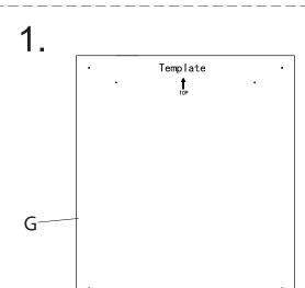
Temporarily secure the paper (G) to the wall, then mark the anchor (H) locations on the wall through the holes. Remove the paper (G) and drill holes making them slightly smaller than the anchors (H) provided.
