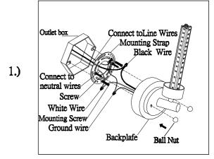
Step.1: Remove mounting bracket from fixture and install to electrical box. Wire fixture to wires in outlet box. Copper wire is for Ground.
