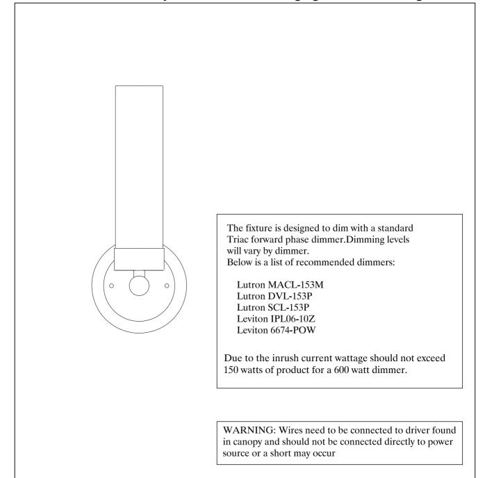
IMPORTANT: Turn off the power at the main fuse or circuit breaker box before starting installation
