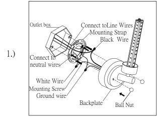
Step.1: Remove mounting bracket (A) from fixture (C) and install to electrical box using screws provided (B). Wire fixture to wires in outlet box. Copper wire is for Ground.
