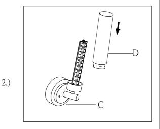
Step.2: Turn the glass (D) onto cup to secure.
