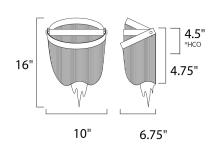
\*height from top of fixture to center of outlet
